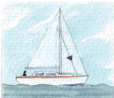
A motor sailing cone is the international day shape indicating that a boat is proceeding under sail when also being propelled by machinery. The motoring cone shall be exhibited forward where it can best be seen, apex downwards. A vessel that is proceeding under sail when also being propelled by machinery is for the purposes of the COLREG, a power driven vessel and should at night display the lights of a power driven vessel.
