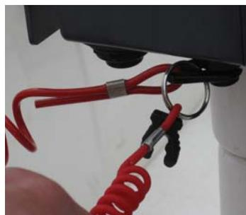
**Locate the kill switch and attach the two lanyards as above**
